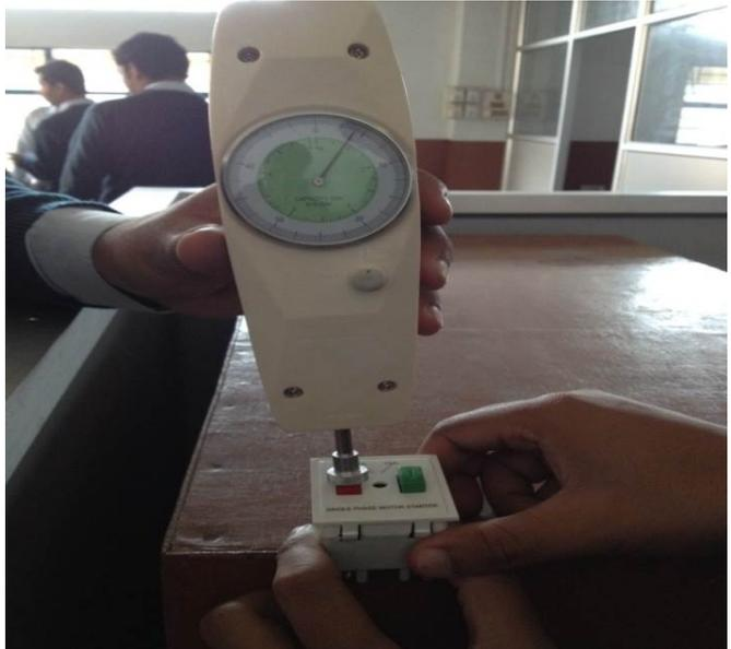
**Fig.8:** Use of force gauge to calculate the force required to switch OFF the starter
