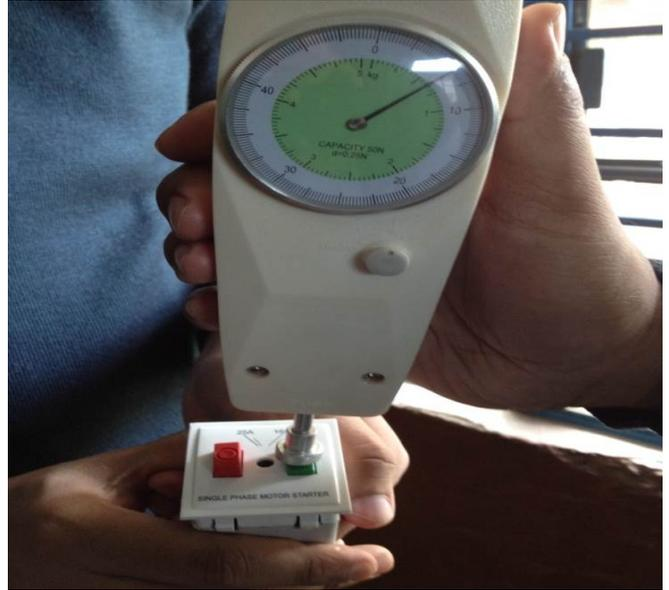
**Fig.7:** Use of force gauge to calculate the force required to switch ON the starter
