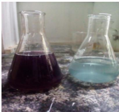
Fig.3.5 wastewater before and after treatment (at 4 mg/L Fe<sup>2+</sup>, 60 mM H<sub>2</sub>O<sub>2</sub>, pH=3, 20 w/ m<sup>2</sup> intensity, 30 min reaction time)
