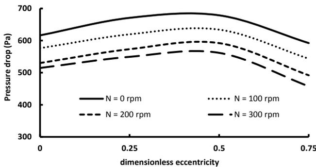
Figure 7 variation of the pressure drop with dimensionless eccentricity using a bit with 4 jet nozzles and  $Re = 1150$
