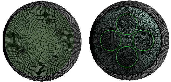
(a) Mesh details at the inlet and outlet. (b) Mesh near the bit nozzles.
