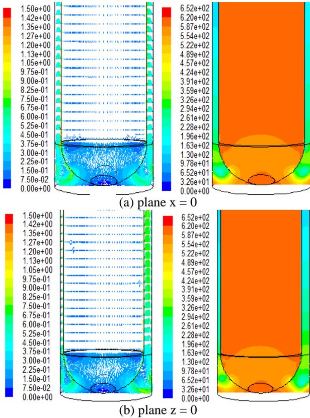
Figure 4 velocity magnitude vectors, m/s (left) and static pressure contours, Pa (right) at  $Re = 1150$  using drilling bit with  $\epsilon = 0.5$ , 4 nozzles and rotating at 200 rpm
