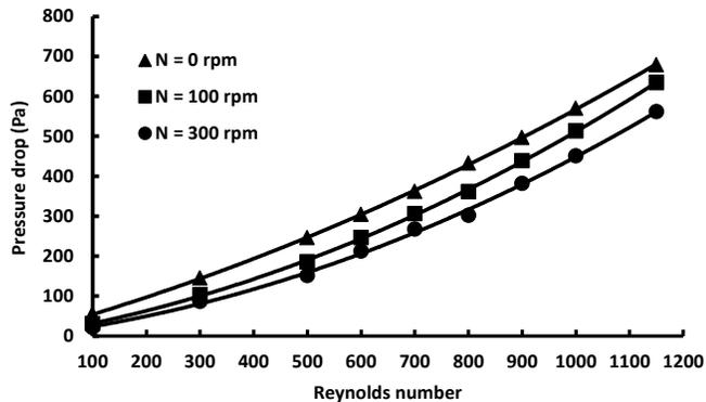
Figure 8 variation of the pressure drop with Reynolds number using drilling bit with 4 jet nozzles and  $\varepsilon = 0.5$ .
