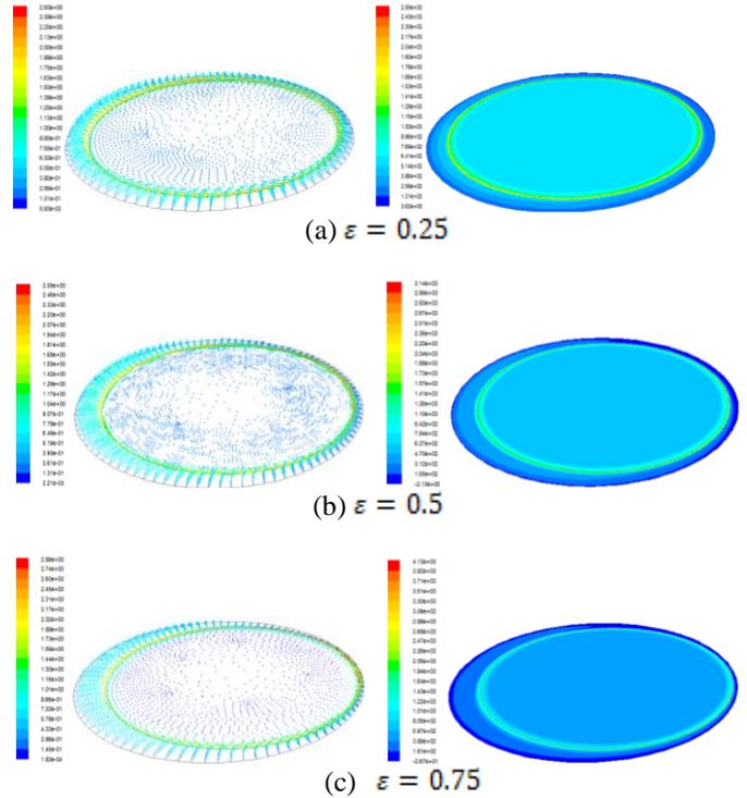
Figure 5 shows axial velocity vectors, m/s (left) and total pressure, Pa (right) in the midway section using drilling bit with 4 jet nozzles and rotating at  $N = 300$  rpm and  $Re = 1150$ .
