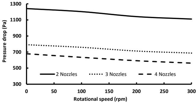
Figure 6 variation of the pressure drop with rotational speed at  $\varepsilon = 0.5$  and  $Re = 1150$
