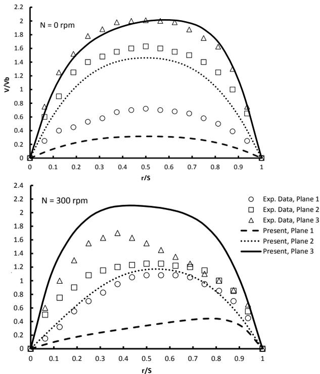
Figure 3 Comparison of numerical and experimental axial velocity profiles at different circumferential planes with  $\epsilon = 0.5$  and  $Re = 1150$  for  $N = 0$  rpm (top) and  $N = 300$  rpm (bottom)
