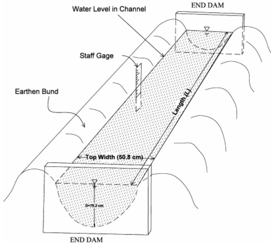
Fig-2 ponding loss measurements
