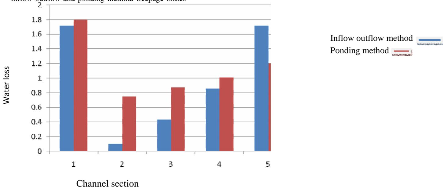
Figure-3: comparison of water loss by inflow outflow and comparison method
