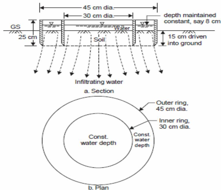
Fig-1 Double ring infiltrometer [12]
