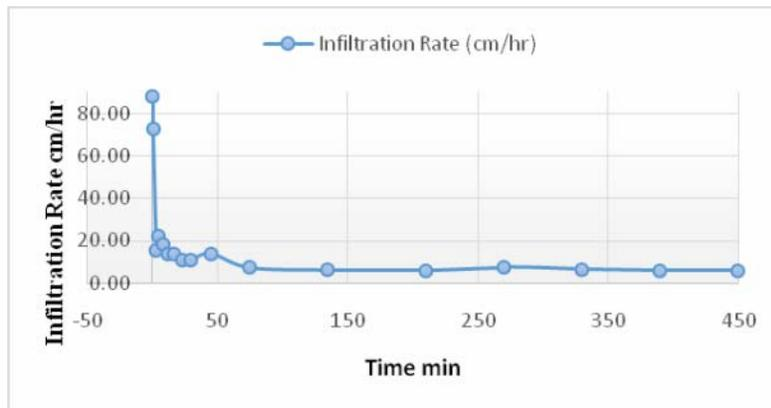
Fig-4 Graph is between Infiltration rate Vs time
