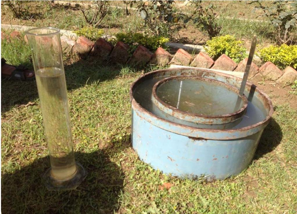
Fig-2 Infiltration Test Equipment
