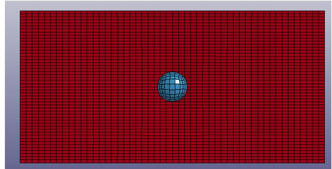
Figure 1. LS – Pre Post model of impactor and plate
