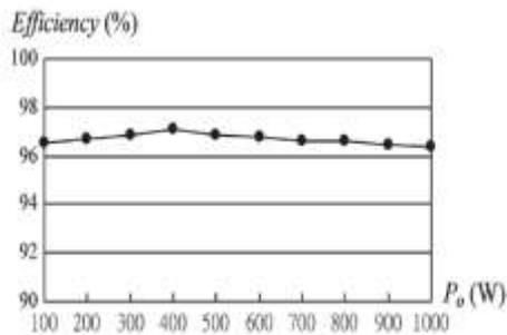
Fig.16 Efficiency of the converter
