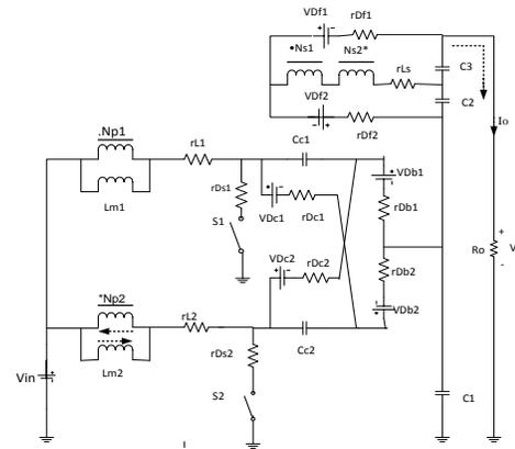
Fig.9 equivalent circuit of proposed converter including conduction losses
