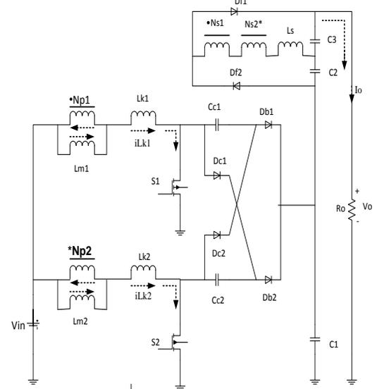
Fig.3 Equivalent circuit of the preferred converter
