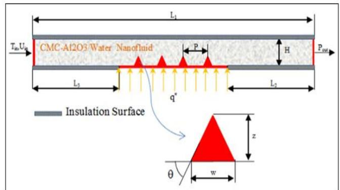
Figure 6. Schematic diagram of experimental setup (Source, [41])
