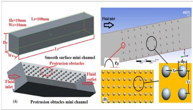
Figure. 9 (A) Domain solution of CFD analysis (B) Protrusion rib parameters(Source, [47])
