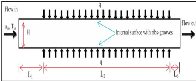
Figure 3. Schematic diagram of rib groove channel (Source, [30])
