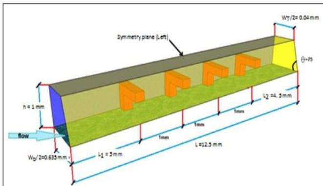
Figure 7. Schematic diagram of experimental setup (Source, [43])
