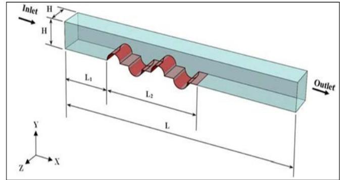
Figure 2. Schematic diagram of 3D arc ribbed grooved passage (Source, [28])
