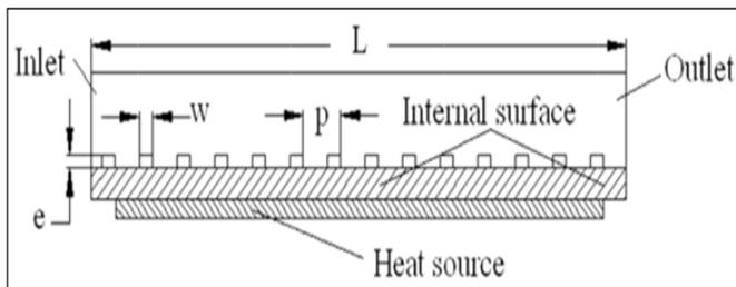
Figure 5. Diagram of channel shape (Source, [37])
