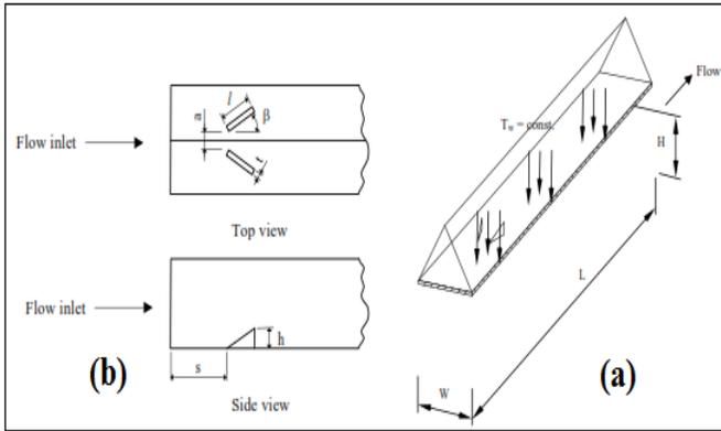
Figure 1. (a) Schematic diagram of problem area, (b) geometric parameters of problem VG (Source, [25])
