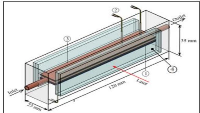
Figure 4. Schematic diagram of rectangular test setup assembly (Source, [35])
